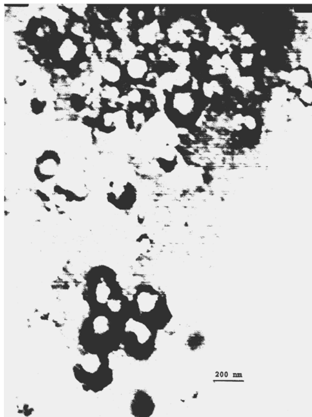
Fig. 4 TEM micrograph of polyacrylamide particles created in supercritical CO 2 , 150 atm and 50 °C, collected on a copper grid using RESS method
